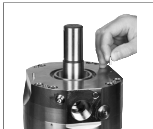
32. Turn pump upside down and mount 2 guide pins.
