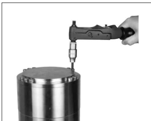
31. Tighten 10 screws to 30Nm.
