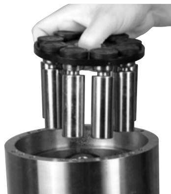
10. Remove pistons and retainer plate.
