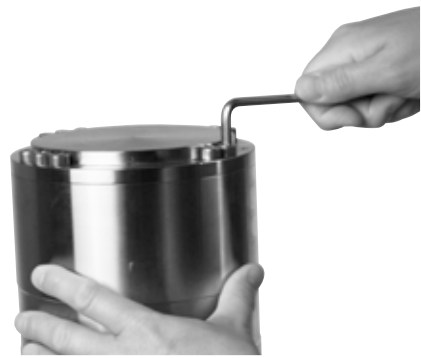
8. Loosen and remove 10 screws.
