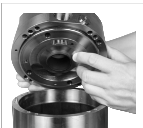
5. Mount port flange on housing. Use pin as guide.
